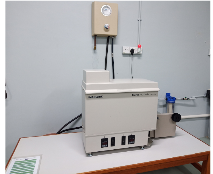
Imagelink Film Processor - for developing microfilm.
