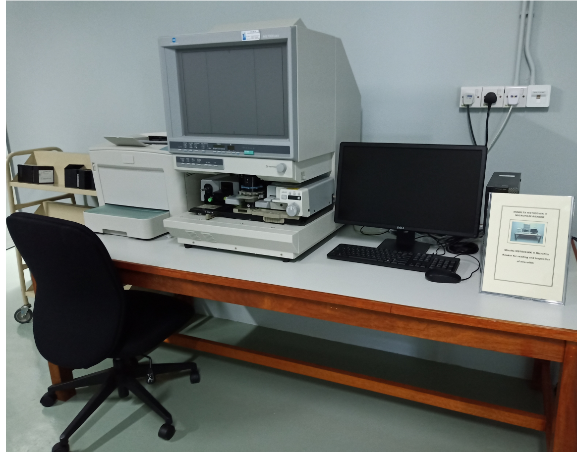
Minolta MS7000-MK II Microfilm Reader - for reading and inspection of microfilm
