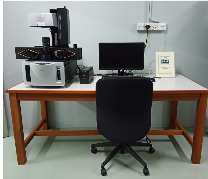
Sunrise Apollo Microfilm Scanner - for scanning of microfilm to digital images.
