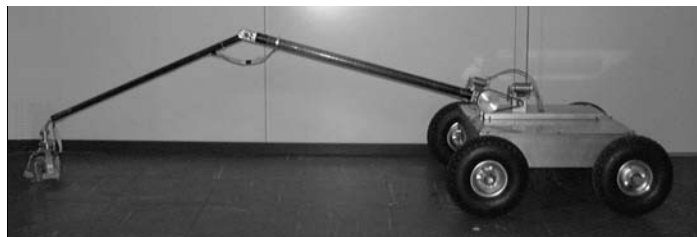
Figure 3 Gripper of Slugbot is designed as far as possible to prevent slime from adhering to the fingers
