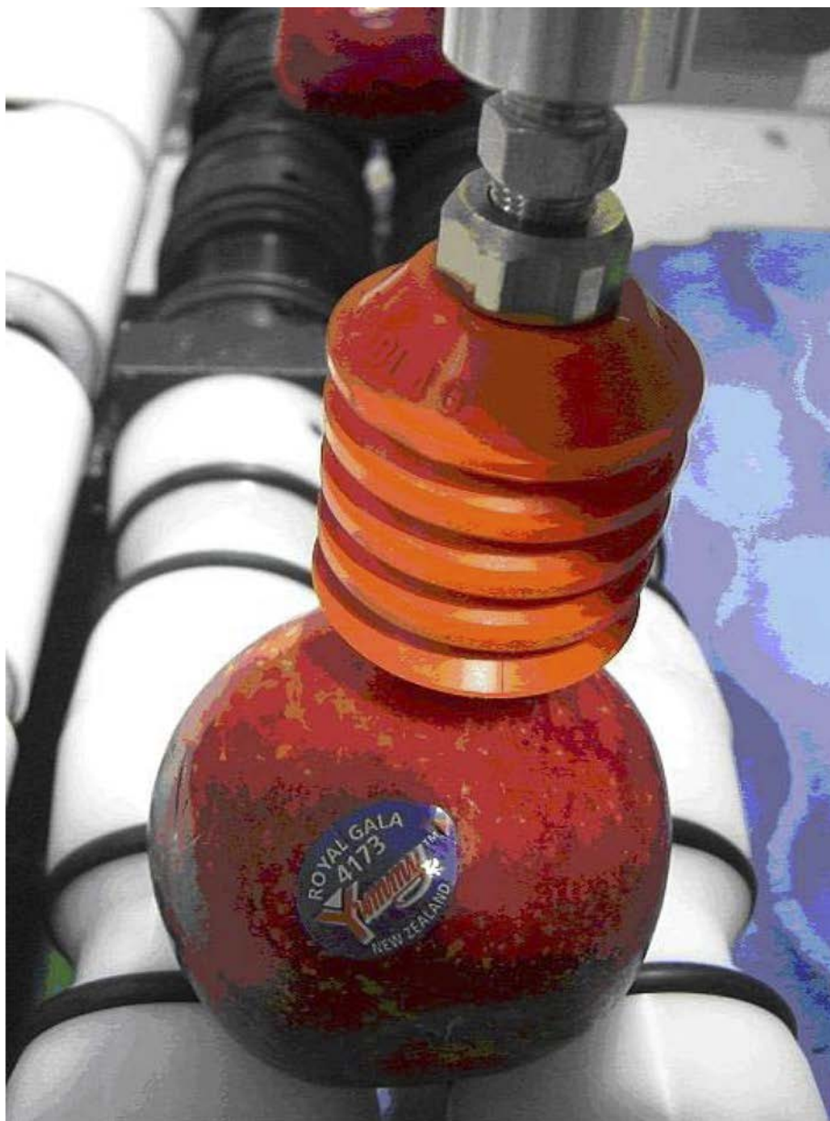
Figure 8 Robotic fruit pickup end of arm vacuum gripper made of soft elastomeric material to handle fruit without bruising during labeling and packing
