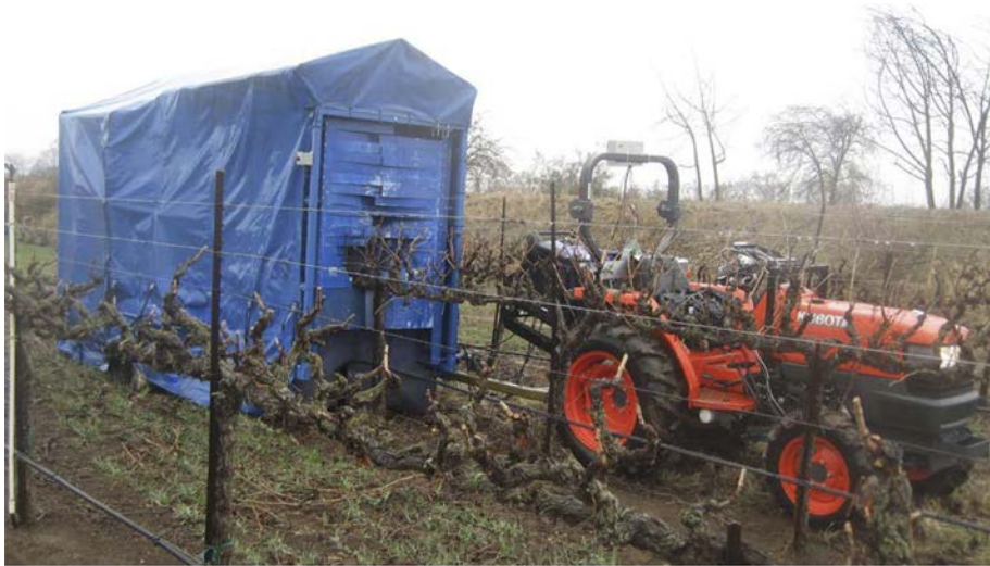
Figure 4 Overall view of tent covered robotic vine trimming system in operation moving down a vineyard row
