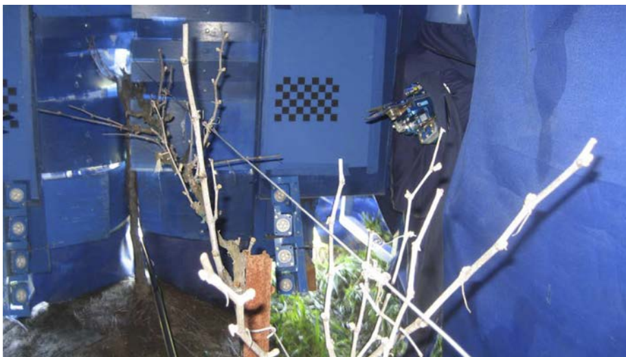
Figure 5 Inside the sun and shadow protecting tent of a robotic vine trimmer in action
