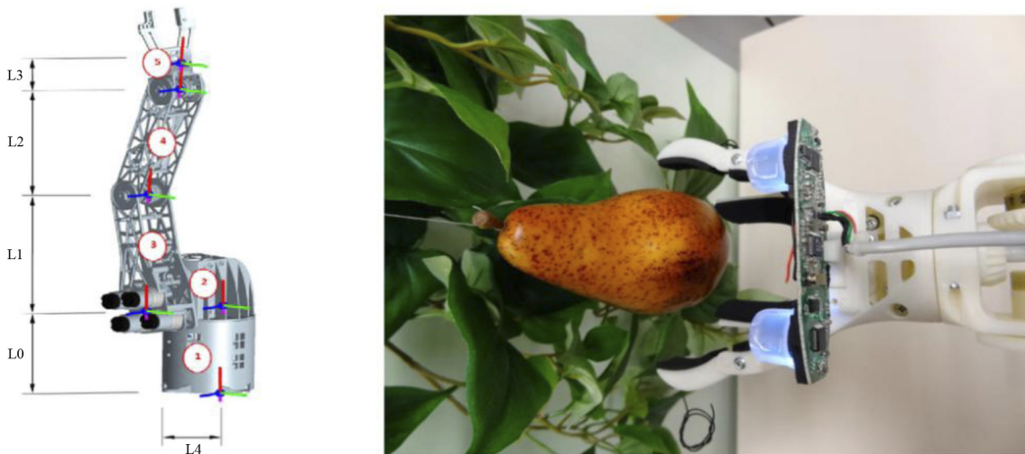
Figure 5 The robotic arm (left); the robot arm-mounted imager and gripper (right)
